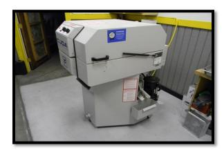
For Sale is a lightly used CUDA 2216 Top Load Series parts cleaner. Rated as industrial, this parts cleaner is easy to use, effective and economical. Some of the highlights: Top Load, Dimensions 42" X 32" X 52", working turntable dia 22", working height 16", 2k heating unit, 23 gal tank capacity, 220v. single phase.
