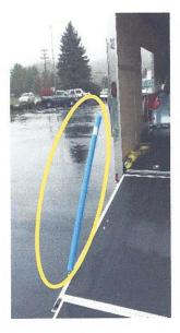
To help guide the car into the trailer and avoid the trailer's wheel boxes, Todd attached a flexible reflector, the type used to mark driveways, on each box's edge. Any tall flexible visible stick/marker will work. They are readily available at local stores.
